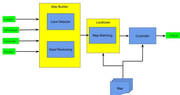
Fig. 1. Architecture for localization in autonomous vehicle
