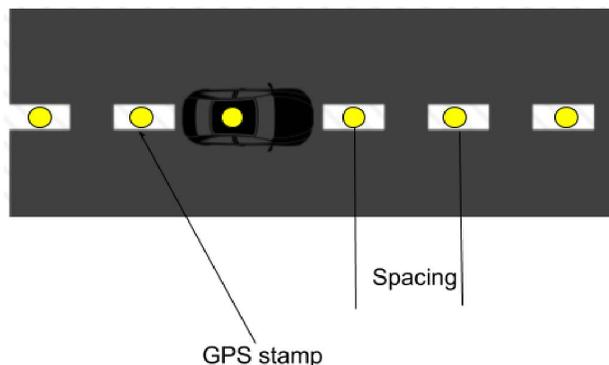
Fig. 3. Lane marking for map generation and positioning
