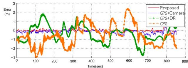
Fig. 5. Lateral localization error: A comparative plot with GPS, Dead Reckoning, Camera and Proposed method
