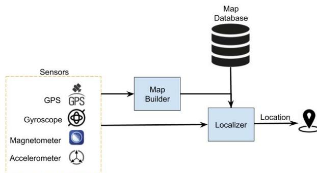
Fig. 2. Sensor data fusion algorithm for localization
