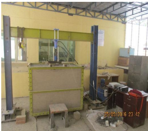
Steel Tank with loading frame
