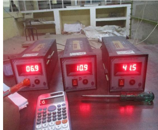
Readout units for load cell and LVDT
